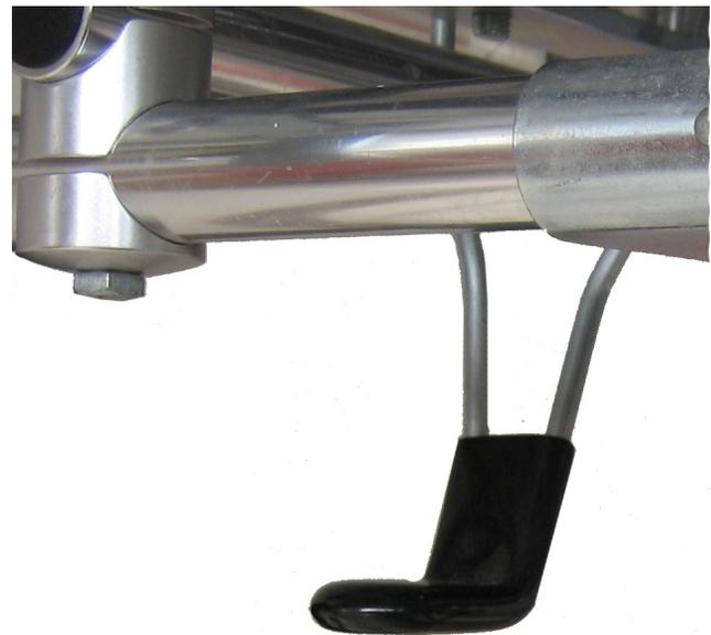
Figure 15 - Leg locking bar
